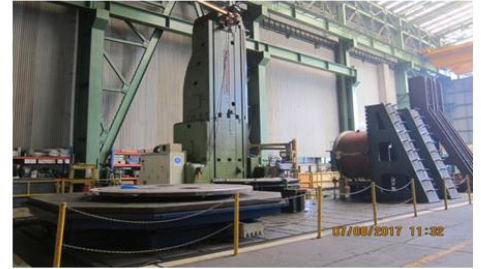
Horizontal Boring Machine - Innocenti mach. capacity: X= 14 m / Y= 6 m / Z= 1.5 m)
