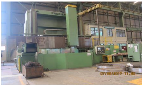
Vertical Turning Lathe - Froriep (mach. capacity: table dia. 4.2 m & height : 4.2 m)
