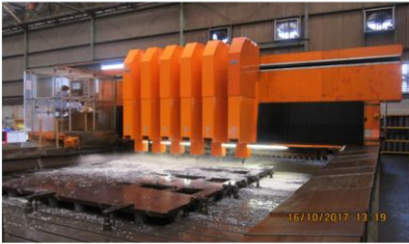
Multi Spindle Drilling and Milling Machine -Georg (mach. capacity: X= 8.5 m / Y= 3.4 m / Z= 550mm)
