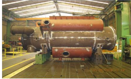
Horizontal Boring Machine - SKODA W200 (mach. capacity: X= 14 m / Y= 3.7 m / Z= 2 m)
