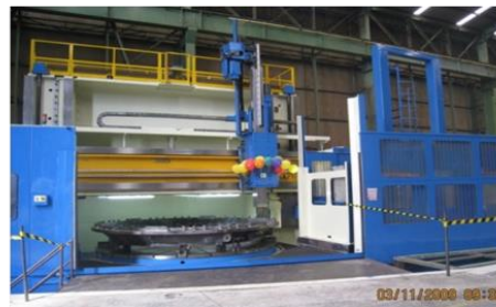
Vertical Turning Lathe - Carnaghi (mach. capacity : table dia. 4.5 m & height: 3.5 m)
